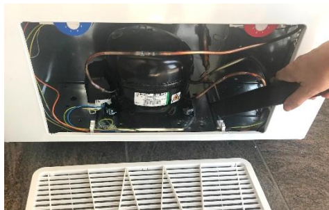
Figure 5 – Cleaning of the compressor room
